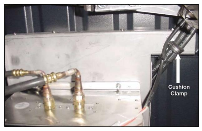
Figure 17. Routing of refrigerent lines.
